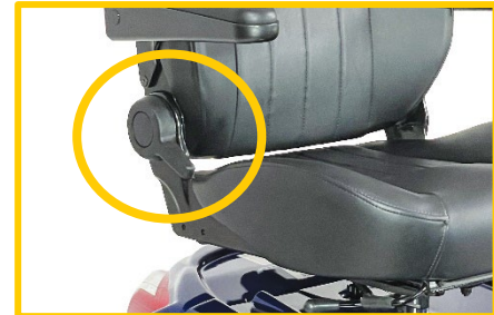
Figure 4 – Pull black handle to adjust the backrest
