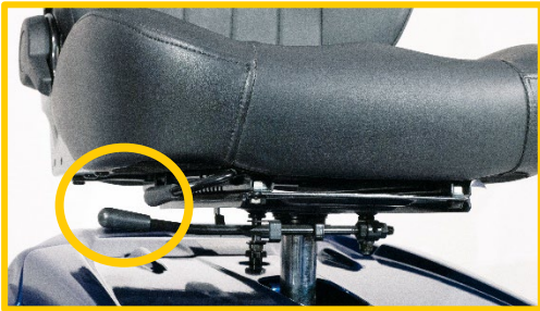
Figure 5 – Pull black handle to control the swivel adjustment
