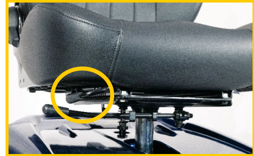
Figure 3 – Lift the handle to adjust the seating position
